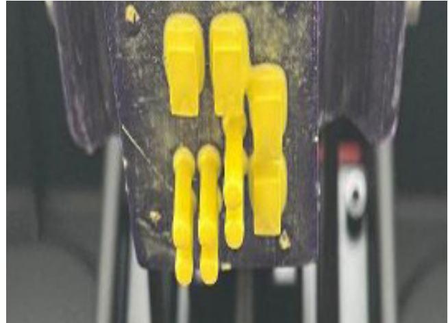
Fig. 5. Printing of ceramic samples from a bone allograft in an Elegoo Mars 4 3D printer
