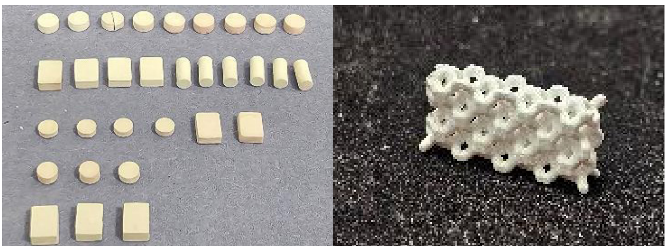
Fig. 6. Ceramic samples from bone allograft after annealing and sintering
