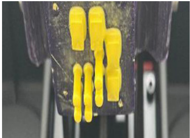
Fig. 5. Printing of ceramic samples from a bone allograft in an Elegoo Mars 4 3D printer
